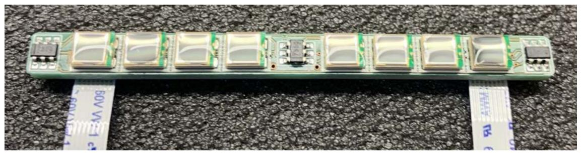
2 readout channels of 4 MPPCs (S13360-3050 PE) by Hamamatsu
